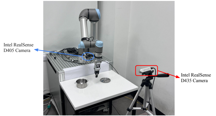
Fig. 7: Real-world robot setup. Our experiments are conducted on a UR5e arm with an RG2 gripper. The observation is captured with a fixed front camera and a wrist-mounted camera, providing complementary viewpoints of the scene for both single-view and multi-view evaluations. All RGB images are resized to 256 \times 256 and the robot is controlled at 10 Hz.
